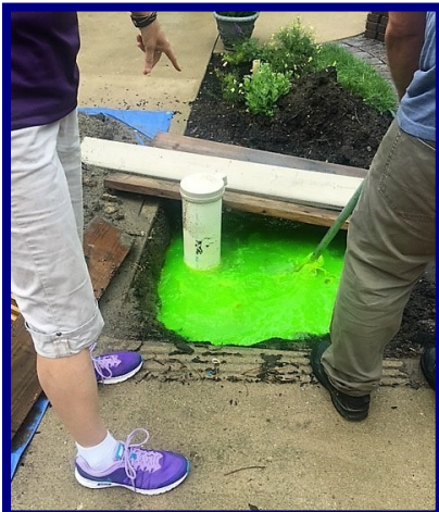
Left: Sanitarians perform a dye test to check the integrity of a well.
