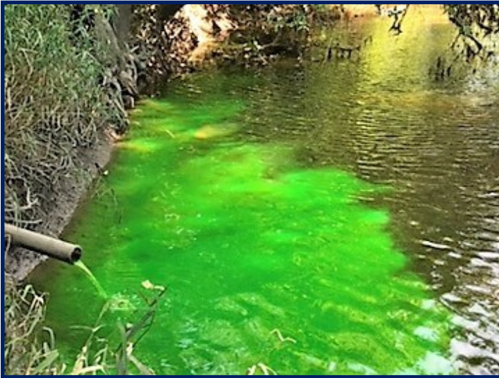
A dye test shows a septic tank draining into a ditch.
